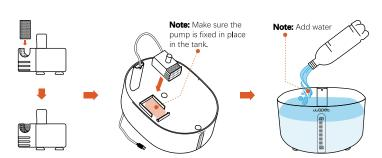
• Install the soaked filter in the filter housing groove Connect flower spout with the bowl lid
