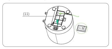
Step 2: Install 3 new D cell, alkaline batteries.(NOT Included)
