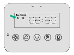
2. Press the  $\bigcirc/\bigcirc$  button to set the "copies". Then press the  $\bigcirc$  button to save.
